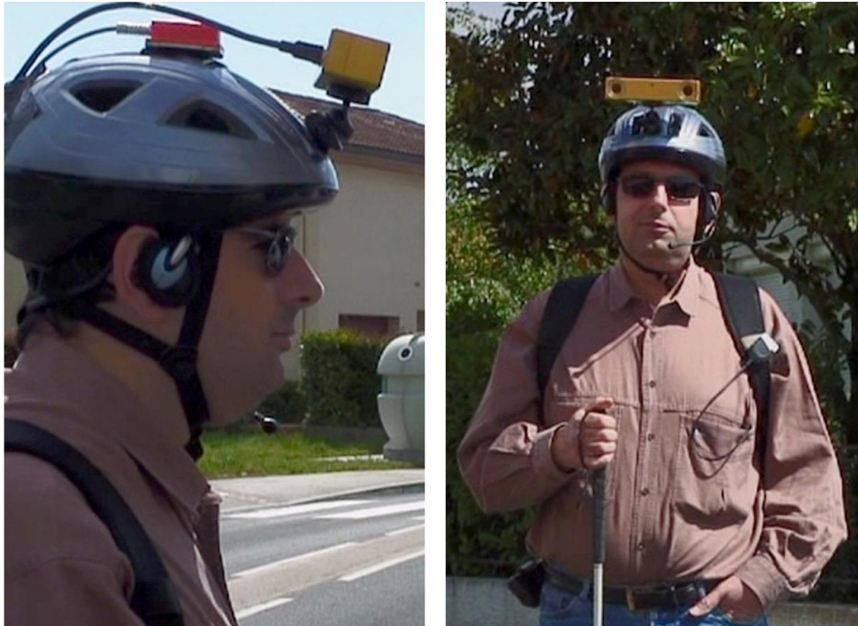
Figure 2 : Bernard Oriola (IRIT) équipé avec le V3 NAVIG prototype. This lab prototype includes a stereoscopic camera, a head-fixed inertial measurement unit, a GPS with IMU attached to the hip, a microphone with stereo headphones (headphones may be replaced with bonephones) and a computer in a backpack.
